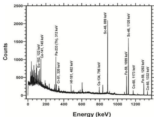
**Fig. 1:** A typical gamma-ray spectrum of an irradiated sediment sample (sample mass 62.2mg, irradiation time 7 min, decay time 1 month, counting time 9000 s)
