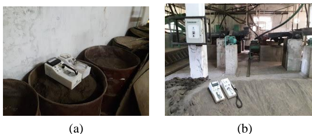
Fig. 3: a) Scintillation radiation survey meter (Model SMGE 12#090202), b) Radiation dose rate meter (Model MDGE 11#101201) and c) Thermoluminescence dosimeter (TLD)
