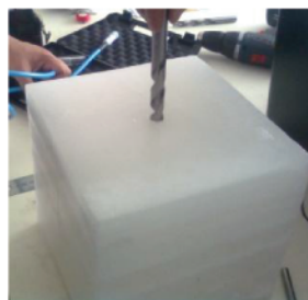
Fig. 3: Preparing hole for ionization chamber insertion
