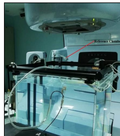
Fig. 2: Phantom setup for PDDs measurements
